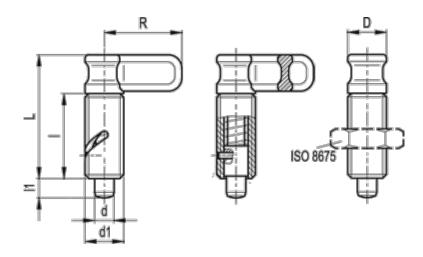
$\begin{array}{lll} D & = 16 \\ d - 0.02 - 0.04 & = 10 \\ d1 & = M16x1.5 \\ I1 & = 8 \\ L \ approx. & = 51 \\ I \ min & = 35 \\ R & = 32 \\ Spring \ pressure \ end \ (N) = 20 \end{array}$
